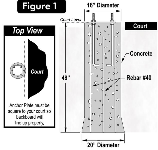
**Note: Using a concrete form for the top 4" of the concrete is recommended. Cardboard forms can be purchased at some hardware and home stores or a wooden form can be constructed out of 2 x 4's.**
