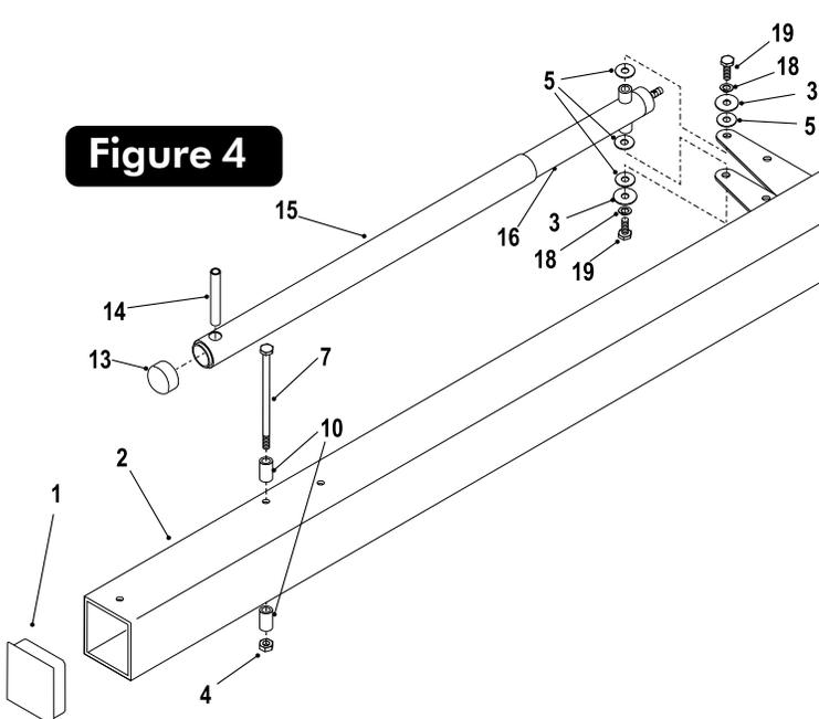
3. Lay Pole (#2) on its side on two padded saw horses. Secure Actuator (#16) to Pole (#2) using one bolt (#19), split lockwasher (#18), washer (#3) and two plastic washers (#5) to thread into each side of Actuator. See Figure 4. Tighten bolts tight.
